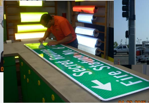
Apply material to aluminum sign backing
